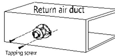
8. Assemble the main unit. Insert the main unit laterally into the air duct's counter interface (left figure) and then rotate it 90° clockwise (right figure). The installation is completed.
