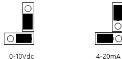
If the range links are incorrectly set, or missing the output range will default to -10 to +40°C
