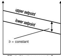
Effect of turning range spindle
