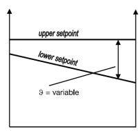
Effect of turning differential spindle
