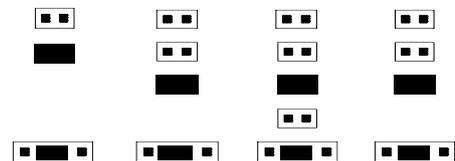
Outputs 1 & 2 are buffered and follow input 1, output 3 follows input 3 and is not buffered, output 4 is adjustable by the pot and is buffered.
